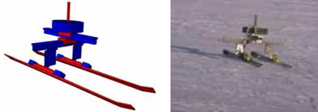
**Fig. 1.** The sledge on skis in the LMS Virtual.Lab software and in the validation experiment.
