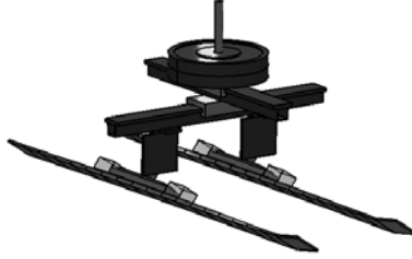
Fig. 1: Model of a sledge on two skis implemented in the multi-body simulation software LMS Virtual.Lab.
