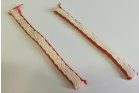
Abbildung 52 New and exposed Mammut Contact Sling (2 months).
