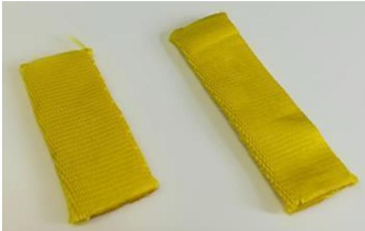
Abbildung 56 New and exposed Nylon slings (2 months).
