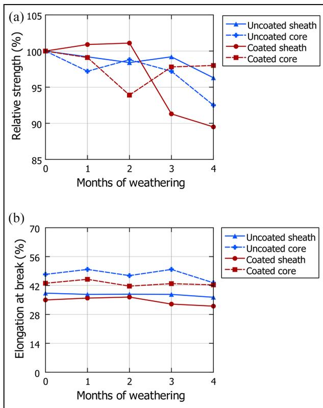
**Figure 7.** Results of the quasi-static tensile test: (a) relative strength calculated from breaking force and (b) elongation at break. Standard deviations are presented in Tables 4 and 5.
