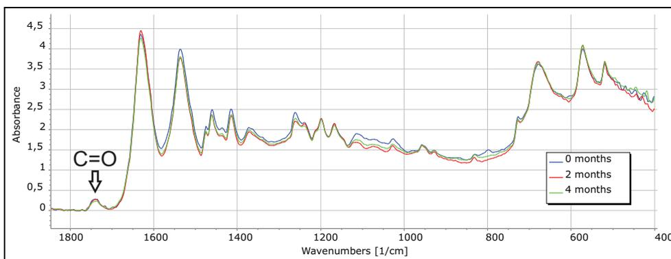
**Figure 9.** Fingerprint region from the FTIR spectra of the coated rope.
