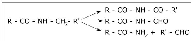
**Figure 2.** Principal overall reactions of the oxidation of polyamides.<sup>19</sup>
