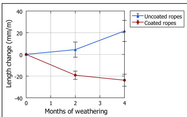
**Figure 10.** Changes in the length of the coated and uncoated ropes due to weathering.
