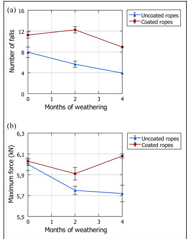
**Figure 6.** Results of the UIAA 101 standard drop test: (a) number of falls to failure and (b) maximum force in the first fall.
