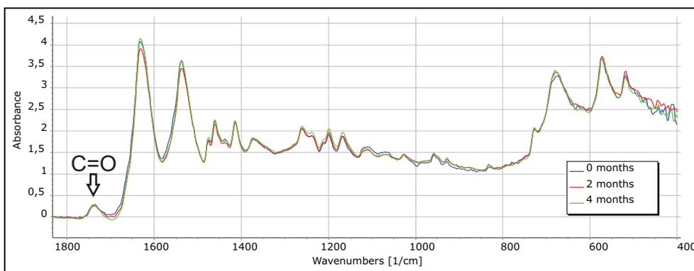
**Figure 8.** Fingerprint region from the FTIR spectra of the uncoated rope.
