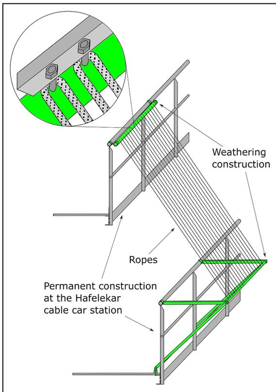
**Figure 3.** Weathering construction and rope placement at the Hafelekar cable car station.
