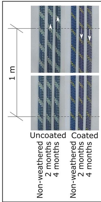
**Figure 5.** Changes in length visible as misalignment of the weave pattern after 1 m.
