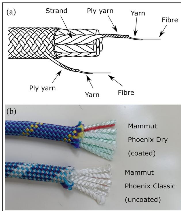
**Figure 1.** (a) Construction of kernmantle ropes and (b) revealed construction of tested ropes.
